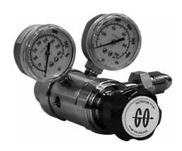
Precision pressure control is now possible with the CYL-20 Series regulator. This two-stage regulator, constructed of 316L stainless steel and PTFE, has less than 0.01 percent outlet pressure change with varying inlet pressures and is designed for use in gas calibration systems and semiconductor materials processing.
