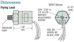
\* Adjustment screw is located under protective screw.
