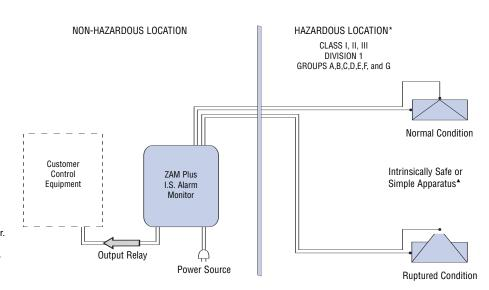
\*Contact ZOOK for information about mounting the ZAM Plus Alarm Monitor in hazardous locations. AHazardous location equipment must be NEC compliant or simple apparatus.
