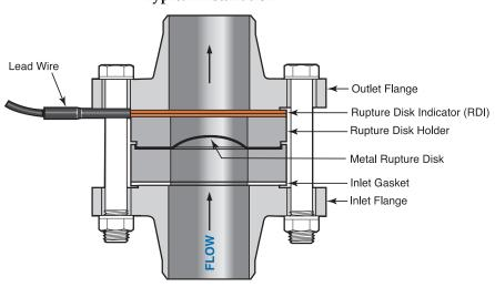
**Note:** RDI is considered a simple device, therefore, approval is not required. Installation must be in accordance with ANSI/ISA RP12.6 and the NEC (ANSI/NFPA 70)
