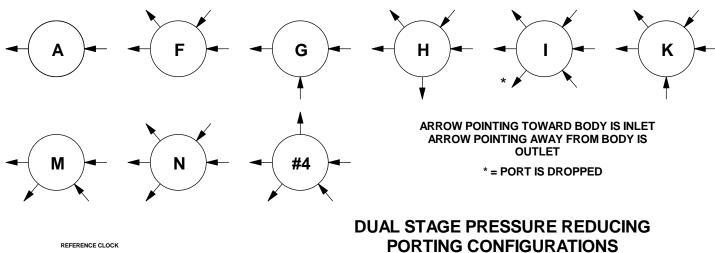
REFERENCE CLOCK 270° 180° 0 90° LOCATION OF PORTS VIEWING FROM TOP OF FIRST STAGE
