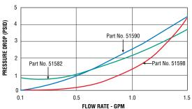
Tests conducted with units in vertical position (lead wires up) with water at  $+70^{\circ}F$  (21  $^{\circ}C).$
