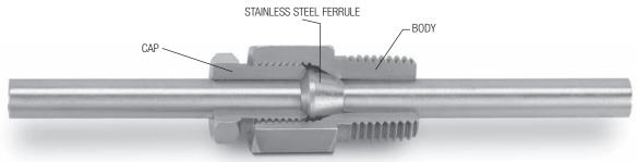
Conax Technologies Model MK Midlock Glands seal a single tube or probe. Featuring a metal-to-metal seal rather than our standard soft sealant technology, MK glands are used where a joint must be opened and resealed in the same setting. Their unique design forms the seal well within the body housing to provide superior performance in high vibration applications.
